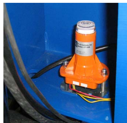
Figure 3-7: Tilt Sensor Adjustment
