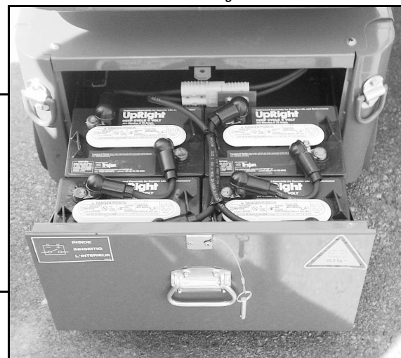
Figure 9: Access to Batteries
