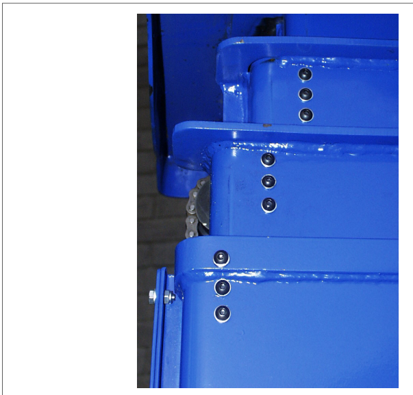
Figure 3-19: Wear Pad Retaining
