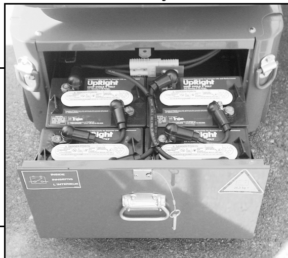
Figure 9: Access to Batteries
