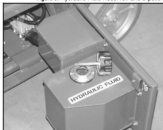
Figure 8: Hydraulic Fluid Reservoir and Dipstick
