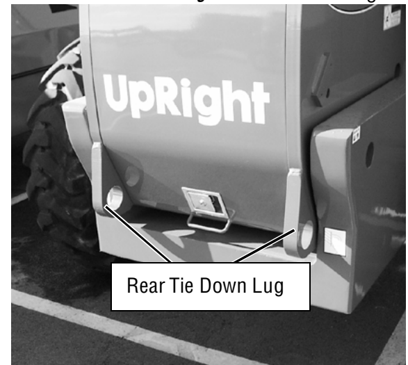
Figure 12: Securing the machine for transportation
