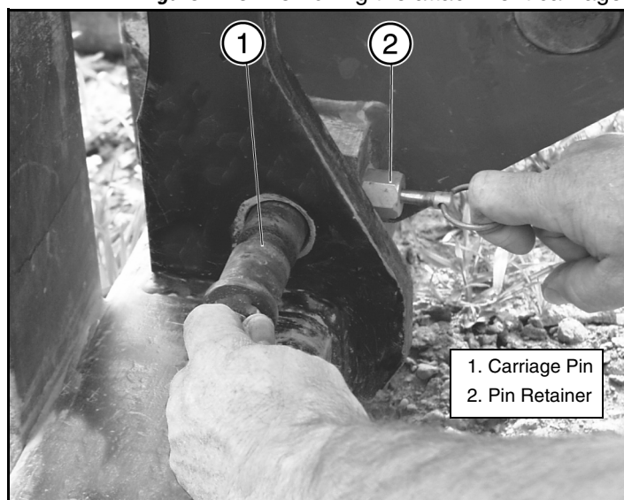
Figure 2-13: Removing the attachment carriage
