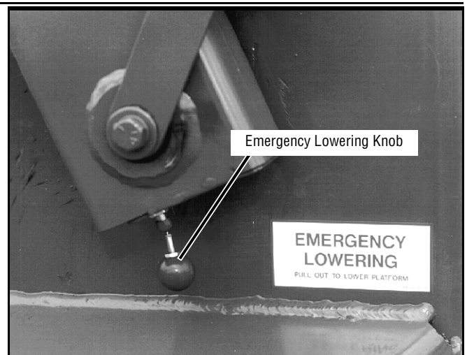
Figure 2-2: Emergency Lowering Knob
