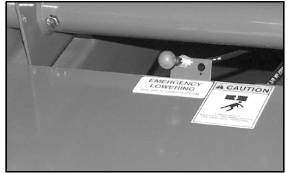
Figure 4: Emergency Lowering Valve,
