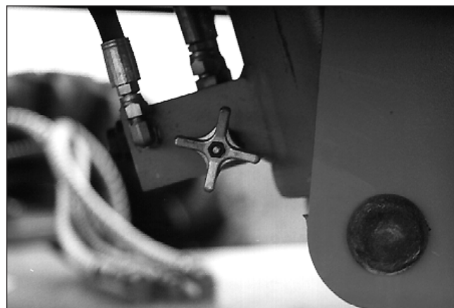
Figure 7 – Emergency Lowering Valve
