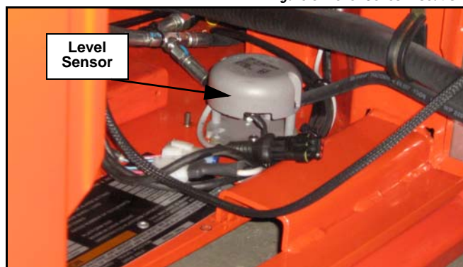
Figure 3: Level Sensor Location
