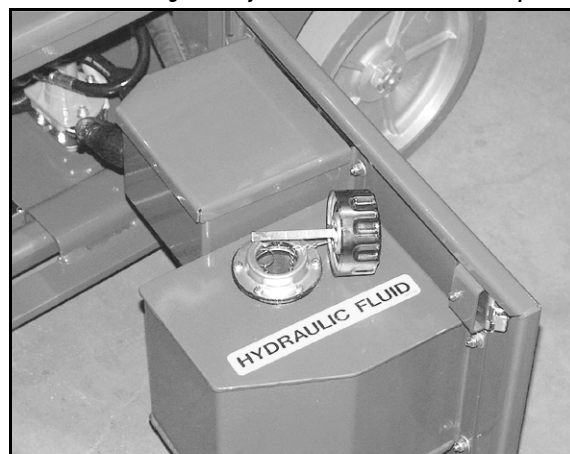
Figure 8: Hydraulic Fluid Reservoir and Dipstick
