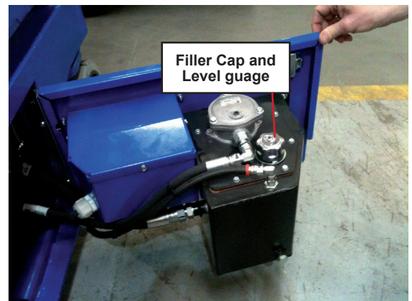
Figure 8: Hydraulic Fluid Reservoir and Dipstick
