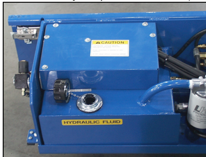
Figure 11: Hydraulic Fluid Reservoir and Dipstick
