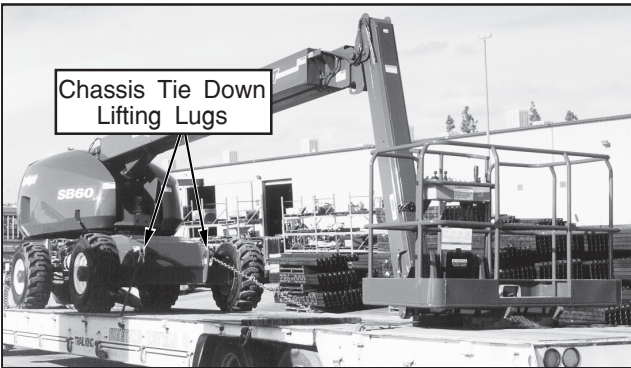
Figure 10: Rear chassis tie down lifting lugs.
