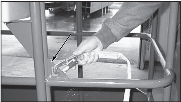
Figure 6: Typical Fall Restraint Anchorage Point
