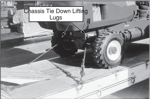
Figure 8: Front chassis tie down lifting lugs.
