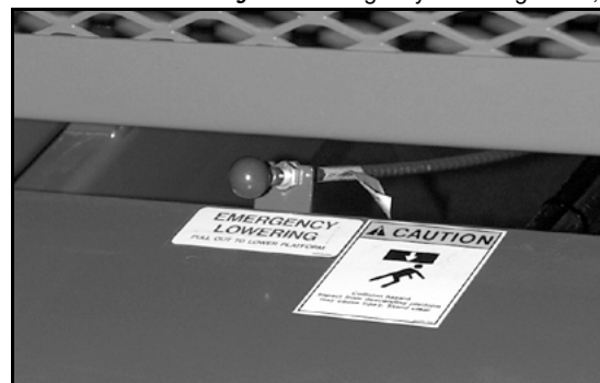
Figure 4: Emergency Lowering Valve,
