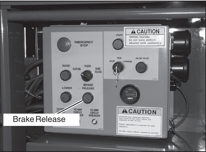
Figure 5: Parking Brake Release
