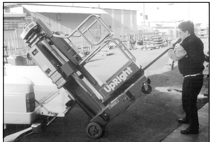
Figure 2-11: Tilting machine onto or off of a vehicle
