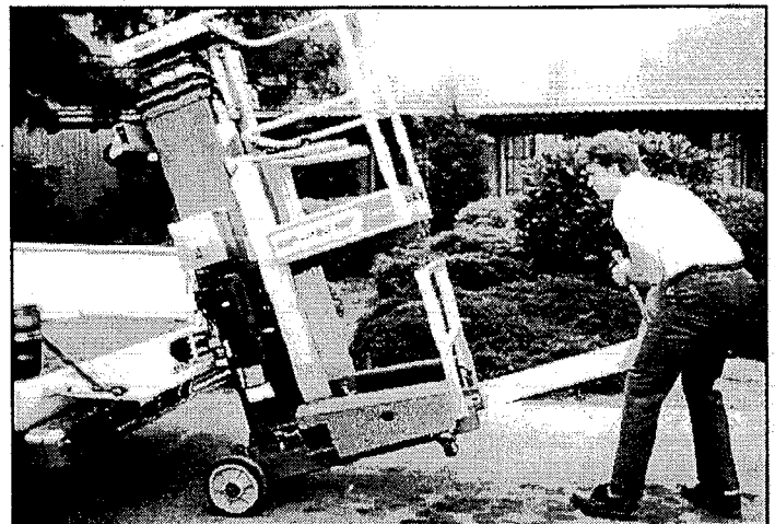
Figure 3-5: Tilting machine onto vehicle
